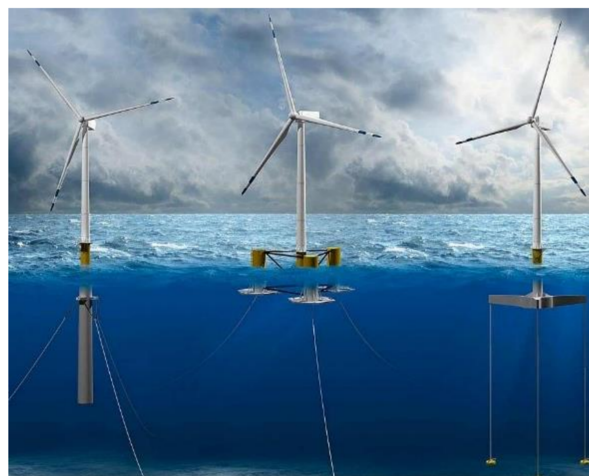
Floating wind power technology types Source: Equinor
