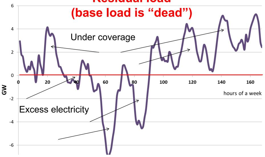
Residual load = Load - non-flexible generation
