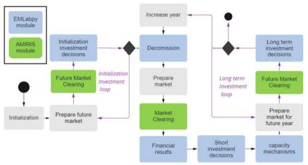
Figure 1 Conceptual workflow of the co-simulation EMLabpy-AMIRIS, which is executed in a yearly loop
